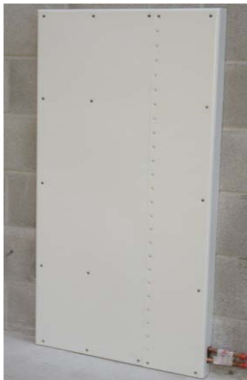
Above, wall mounted NOMS panel before being repeatedly beaten with a four foot long scaffolding pole.
