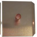
Two 22mm copper tubes mounted in aluminium fins measuring 111 mm x 111mm.
