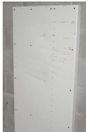
Left , wall mounted NOMS panel before being repeatedly beaten with a four foot long scaffolding pole.
