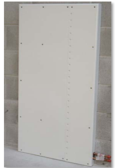
Above, wall mounted NOMS panel before being repeatedly beaten with a four foot long scaffolding pole.
