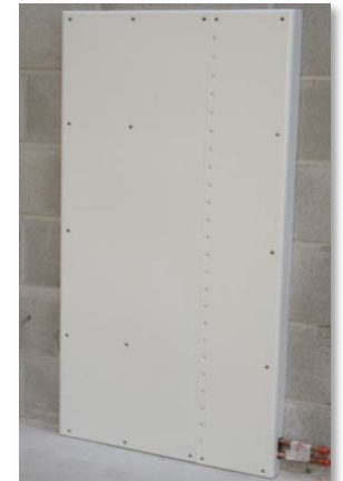
Left , wall mounted NOMS panel before being repeatedly beaten with a four foot long scaffolding pole.
